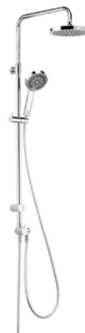
6609105-00 KLUDI A-QA Dual Shower System DN 15 pomme de douche Ø 200 mm douchette A-QA s et flexible Suparaflex 1 600 mm
