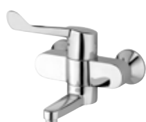
349220524 mitigeur de mural DN 15 levier CLINIQUE bec orientable ou blocable raccords S saillie 180 mm 349200524* saillie 245 mm 349240524* saillie 335 mm
